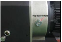
Inspection hole with G1" plug: Check the coupling and its insert, and fan through this hole regularly. (The endoscope(WireCam) can be used with Smart Phone software)
